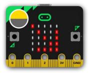
What is it? By reversing the LEDs of the screen to become an input, the LED screen works as a basic light sensor, allowing you to detect ambient light.
