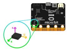
What is it? An accelerometer measures the acceleration of your micro:bit; this component senses when the micro:bit is moved. It can also detect other actions, e.g. shake, tilt, and free-fall.
