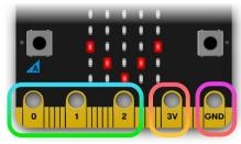
What is it? There are 25 external connectors on the edge connector of the micro:bit, which we refer to as 'pins'. Program motors, LEDs, or other electrical components with the pins, or connect extra sensors to control your code!
