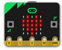
**What is it?** LED stands for Light Emitting Diode. The micro:bit has 25 individually-programmable LEDs, allowing you to display text, numbers, and images.
