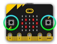
**What is it?** There are two buttons on the front of the micro:bit (labelled A and B). You can detect when these buttons are pressed, allowing you to trigger code on the device.
