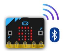
What is it? BLE (Bluetooth Low Energy) allows the micro:bit to control phones and tablets over Bluetooth. This communication works both ways, so you can also send code to your micro:bit wirelessly from your phone <u>using one of our apps</u>. Other apps, such as Swift Playgrounds and Scratch, use Bluetooth to talk to the micro:bit.
