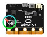
What is it? The compass detects the earth's magnetic field, allowing you to detect which direction the micro:bit is facing. The compass has to be calibrated before it can be used.
